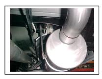
INSTALL BAND CLAMP # F ONTO MUFFLER, INSERT HANGER INTO RUBBER GROMMET, USE BOLT KIT #H PROVIDED, DO NOT TIGHTEN.
