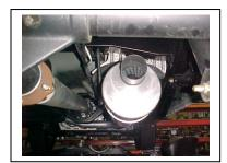
INSTALL MUFFLER # C ONTO YOUR RESONATOR 1 ½" –2". USE CLAMP #G TO SECURE MUFFLER TO THE PIPE, DO NOT TIGHTEN. OUTLET WILL BE AT THE 12 O'CLOCK POSTION. INLET WILL BE LOOKING INTO LOUVERS.
